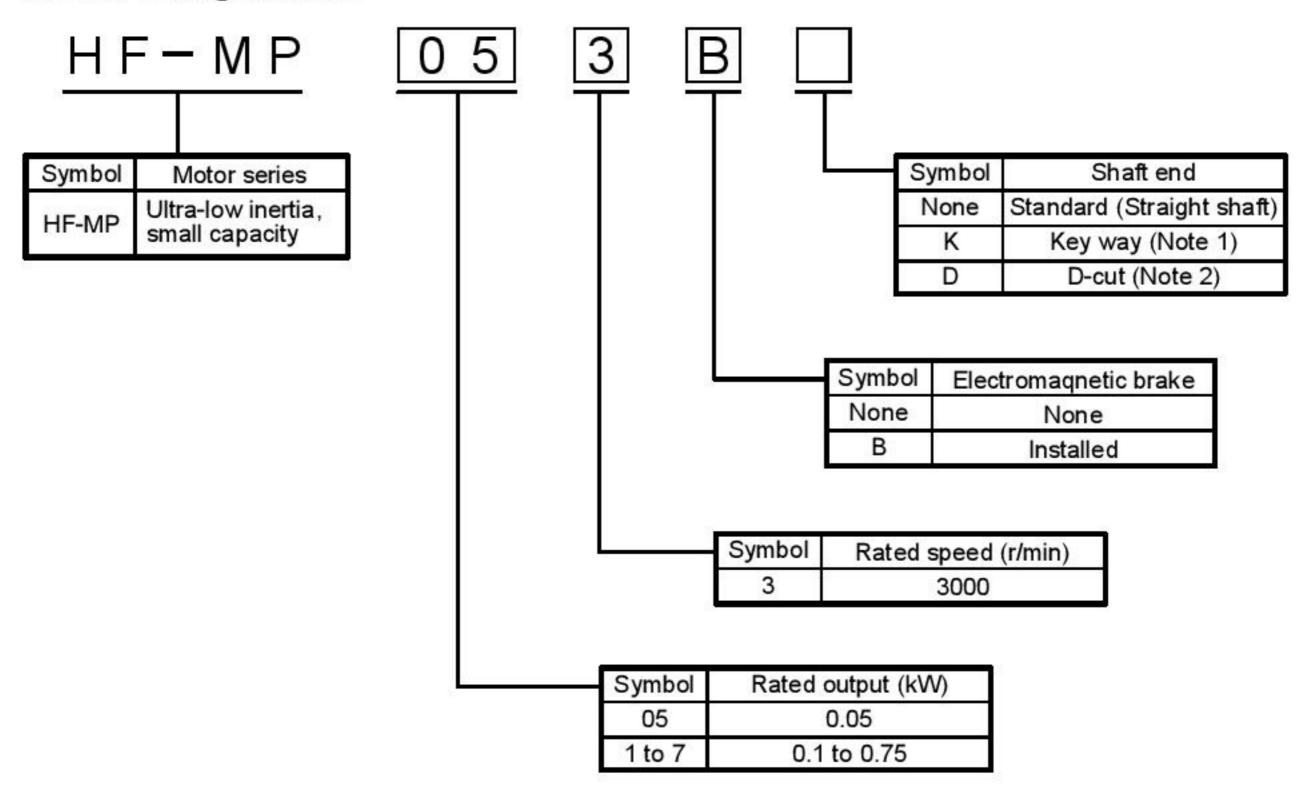
Notes: 1. 200W or larger capacity HF-MP ☐ K has a key. 2. D-cut is available for 100W or smaller capacity.
